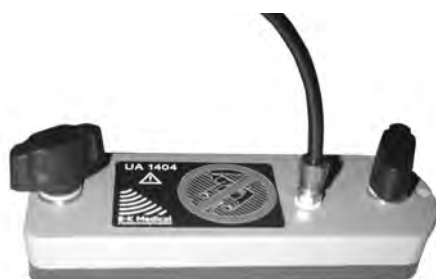
Figure 6. UA1404 – Black screws to attach the lid to the plug.
